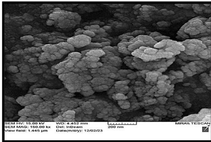
**Fig 3.** FESEM micrograph of turmeric nanoparticles spherical well scattered with a size average of 49.8 nm.
