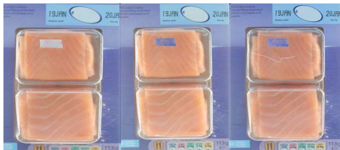
Fig. 8 – Left: before UV activation, middle: after UV activation and right: on opening the packages.
