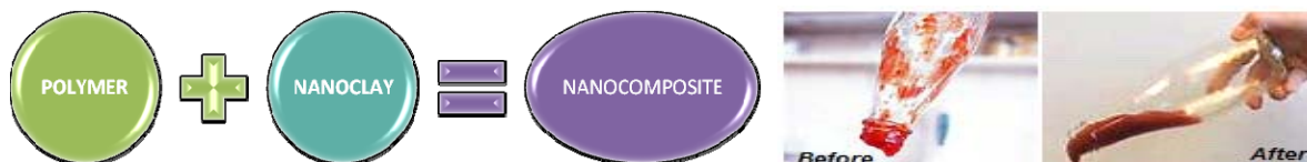
Fig. 6 - Non-Stick nano food packaging for mayonnaise and tomato sauce bottles. ( http://www.fastcoexist.com/1679878/mits-freaky-non-stick-coating-keeps-ketchup-flowing ).
